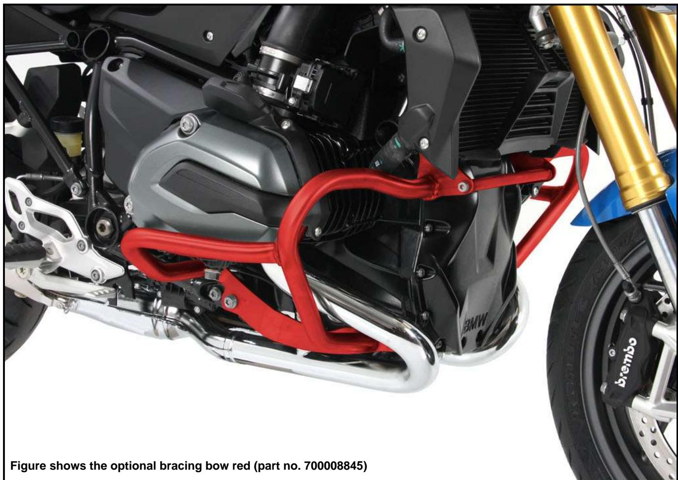
Figure shows the optional bracing bow red (part no. 700008845)
